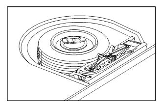
Lift and remove the cover. See "Compact Spare Tire" later in this section for more information about the compact spare.
